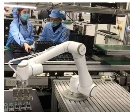
Pick & place of PCB boards
