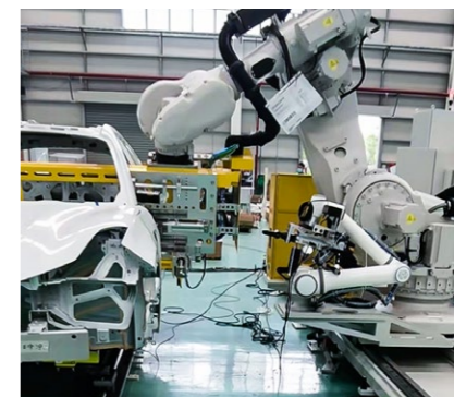
Screwing car body parts
