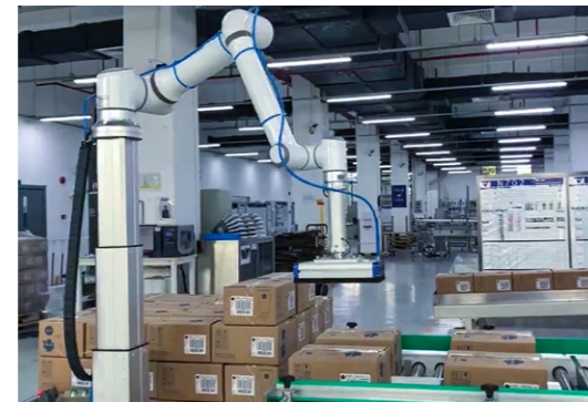
Palletizing with lifter and gripper extender
