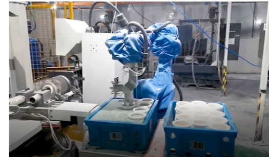
Salt cores pick & place with vision system
