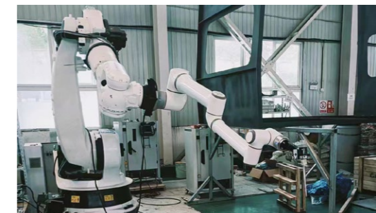
Integration with industrial robot for bus body painting
