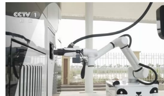
Electric cars fueling with AGV
