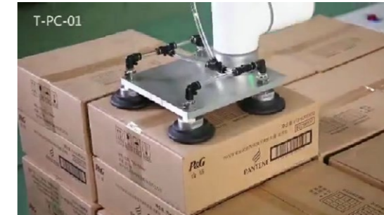
Palletizing in the FMCG industry at P&G plant
