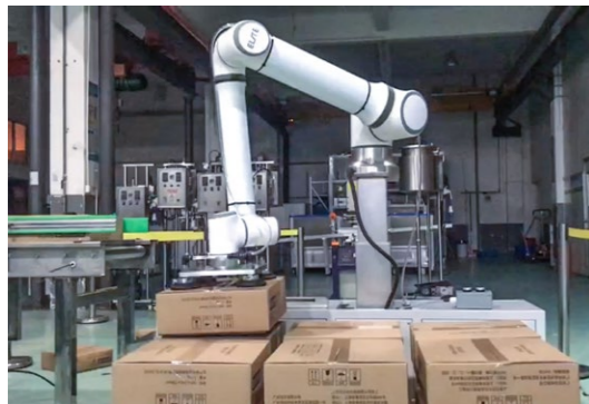
Mid-payload palletizing with lifter
