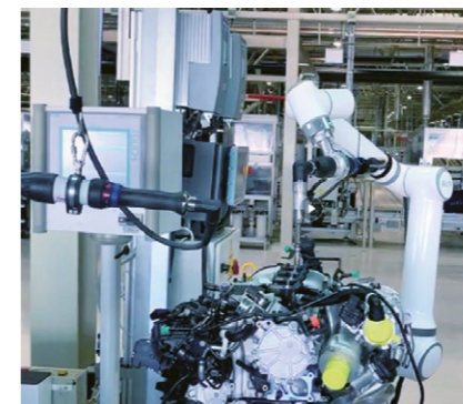
Tightening of engine bolts
