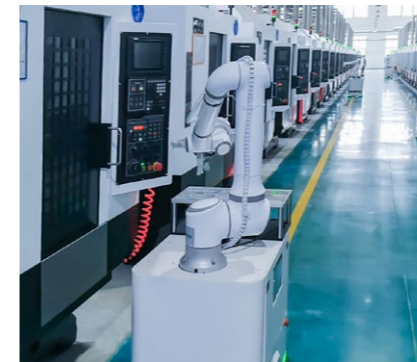
CNC machine tending with AGV
