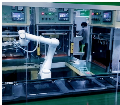
1-to-3 pick and place with machine tending
