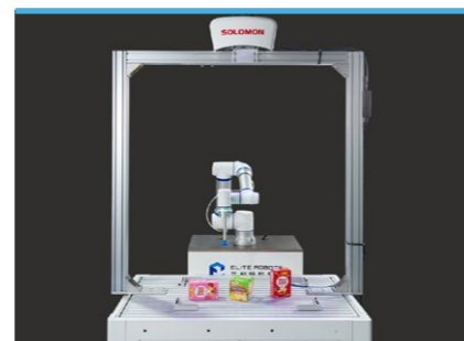
Sorting solution with Solomon 3D camera
