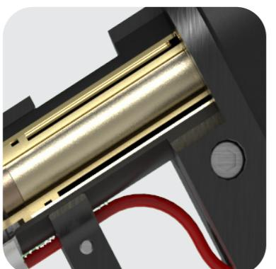
**Better cooling.** Powerful cooling circuit up to the diffuser
