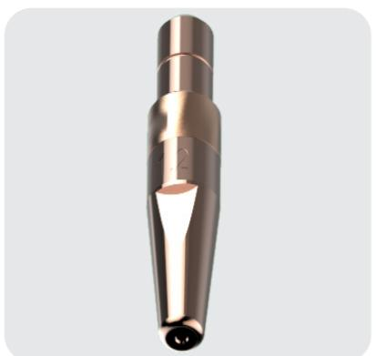
M10 contact tips with long length and high resistance BICOMP materials, triple the life of a standard tip.
